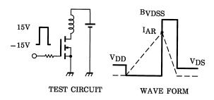
$$\begin{aligned} &R_G = 25~\Omega \\ &V_{DD} = 90~V,~L = 24.5~mH \end{aligned} \qquad E_{AS} = \frac{1}{2} \cdot L \cdot I^2 \cdot \left( \frac{BVDSS}{BVDSS - VDD} \right) \end{aligned}$$
